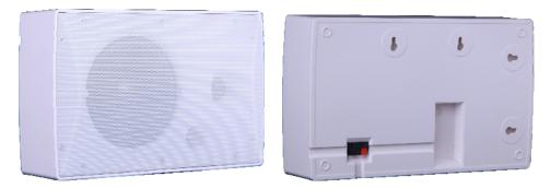
Active Bluetooth wall mount speaker, made of ABS body and arc design metal grill, with 2-way 4 inch woofer and 1 inch tweeter, rated power 12-15 Watts, use for small rooms or hotel rooms. Fast installation with screws on wall. It is delivers clear sound and practical use at very competitive cost to satisfy medium or high level sound system.
