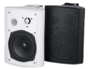
Wall mount speaker, designed in ABS material, 4 inch, 5 inch, 6 inch woofer and 1 inch tweeter speaker, rated power 20W, 30W and 40 Watts, use for commercial audio system or public address system (pa system) of input voltage 100 volt or power switch to 1/2, 1/4 power and  $8\Omega$ . Fast installation with strong mounting bracket. It is durable and practical and very competitive to satisfy sound system at economical budget.
