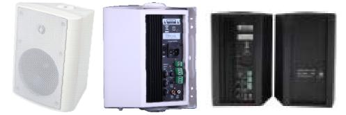
Active wall mount speaker, designed in ABS body, with a 2-way 5 inch/ 6 inch speaker, built-in amplifier rated power 25/35 Watts @  $8\Omega$ , use for home audio system or public address system (pa system). Fast installation wall mounting bracket and angle adjustable. Treble, bass and master volume control, balance phoenix / RCA and 3.5mm input. The speaker also can be used for home audio system. It is durable and practical and very competitive to satisfy medium or high level sound system.
